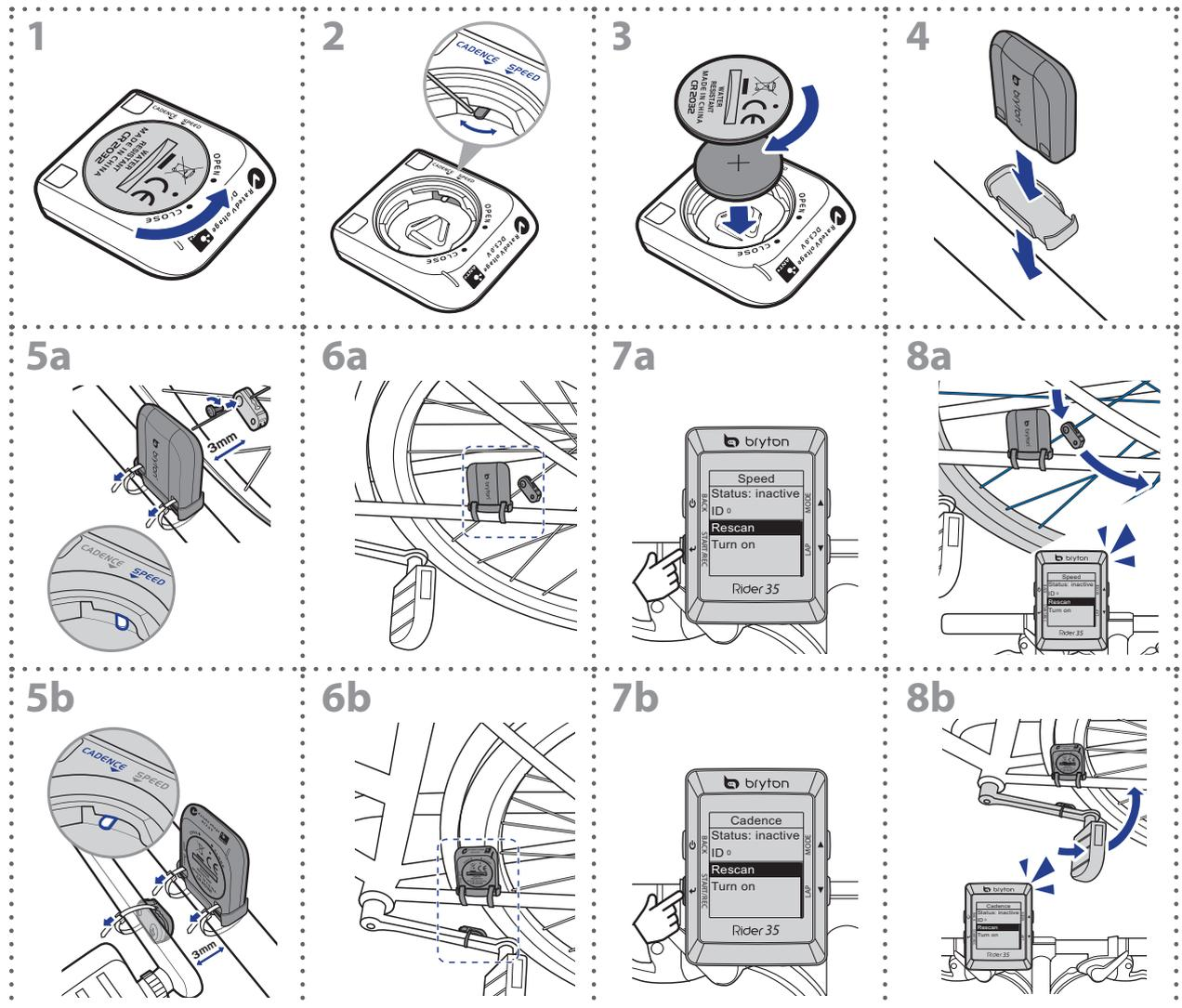
**NOTE:** To ensure optimum performance, the distance between the sensor and the magnet must be within 3 mm.
