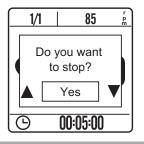
**NOTE:** When recording, press 5/=/= twice to stop recording.
