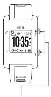
Press and hold these 2 keys to force a system RESET.
